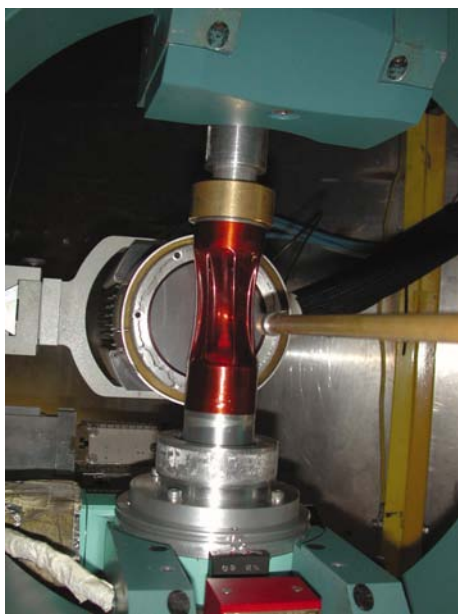
Figure 1 Huber four-circle diffractometer at beamline D3 (HASYLAB) equipped with He cryostat and Smart 1K CCD area detector. The vacuum chamber wall at the cold head of the cryostat is made of Kapton film.
